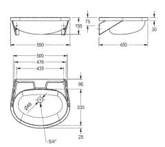
Single wash basin for wall mounting, stainless steel, surface satin finished, material thickness 1 mm, seamless welded bowl with diameter  $500 \times 335 \times 155$  mm, oval shape, 90 mm tap ledge, prewelded mounting brackets, with soap dish, includes screws and dowels.
