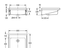
A single bowl sink manufactured from 1.2 mm thick, grade 1.4301 (304) stainless steel, satin polish finish. The sink top is turned down on all four edges and incorporates a wet area recess. The bowl is prepared for a 38 mm waste outlet.
