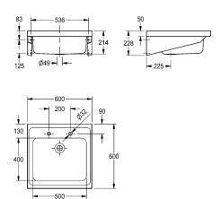
A single bowl sink manufactured from 1.2 mm thick, grade 1.4301 (304) stainless steel, satin polish finish. The sink top is turned down on all four edges and incorporates a wet area recess. The bowl is prepared for a 38 mm waste outlet.
