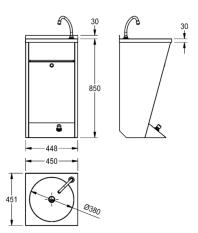
Single wash basin, floorstanding, wall mounting, stainless steel, surface satin finished, material thickness 1 mm, seamless welded round bowl with diameter 380 mm, rectangular shape, 35 mm tap ledge, without overflow, 1 1/4" plug waste, drainage centric, incl. premounted spout, floor standing trap cover with premounted self-closing valve for foot operation, water temperature adjustable with valve, front cover can be removed, includes screws and dowels.
